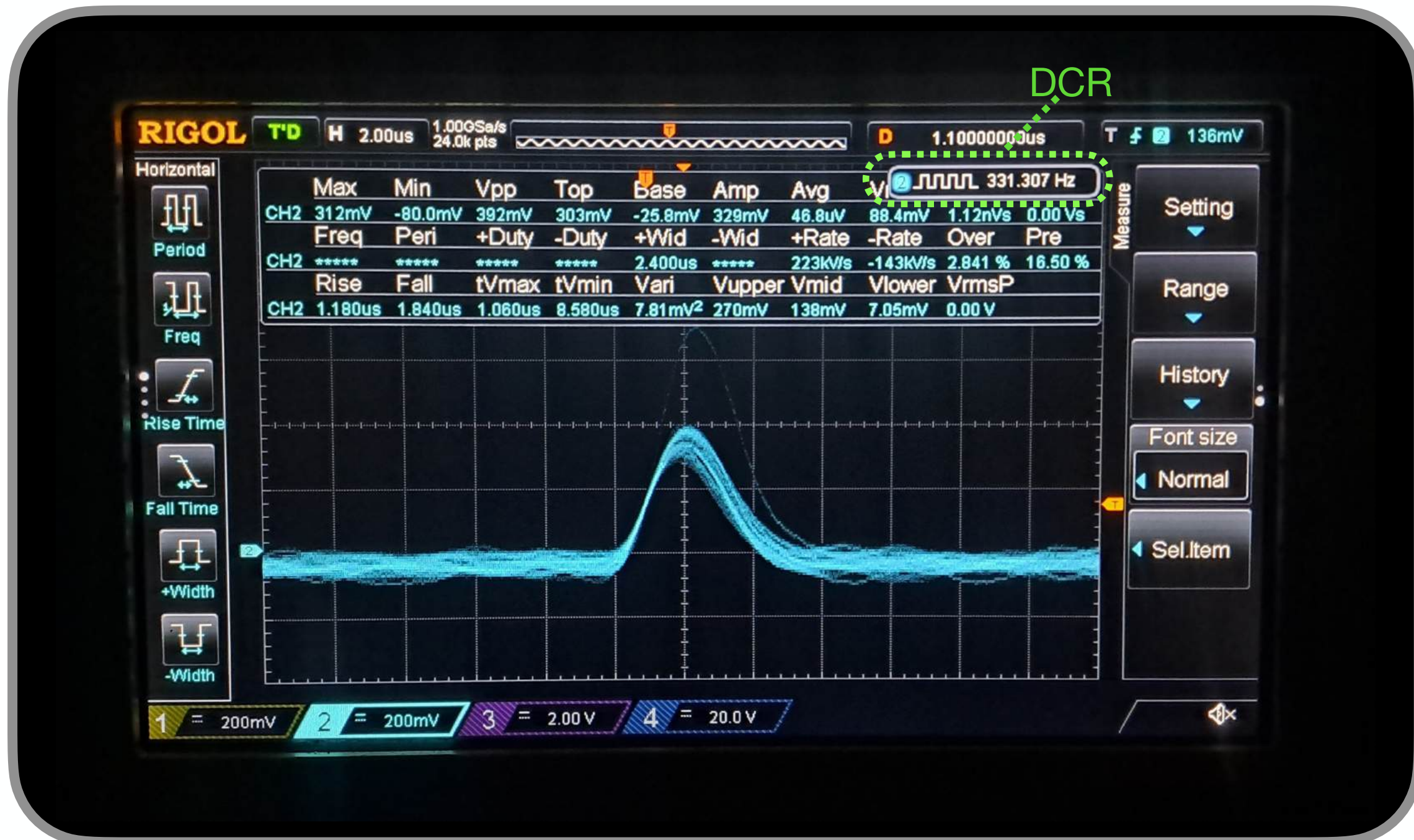
Single Photon Counting through SiPM pulse mode testing
